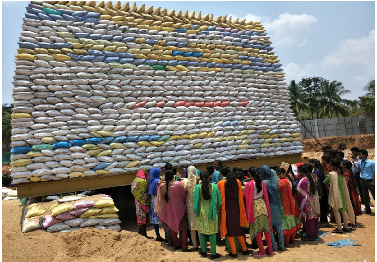
Dr. O. Eswara Reddy explaining the Testing Procedure of Pile Load Test
