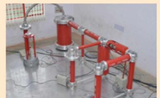
100 kV High Voltage Testing Equipment
