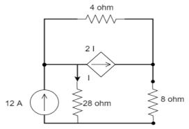
M1Q3. Find node voltages V1,V2 and V3 using node analysis for the circuit shown in the figure.
